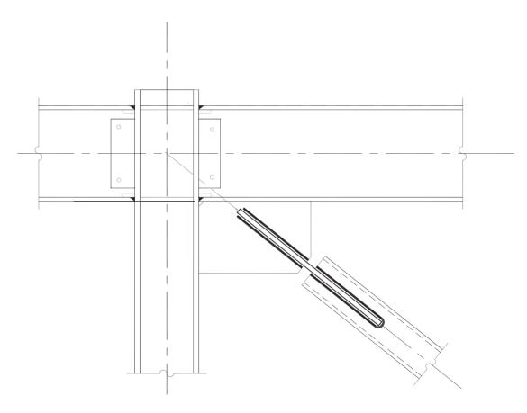
Figure 2-3. Typical gusset configuration
